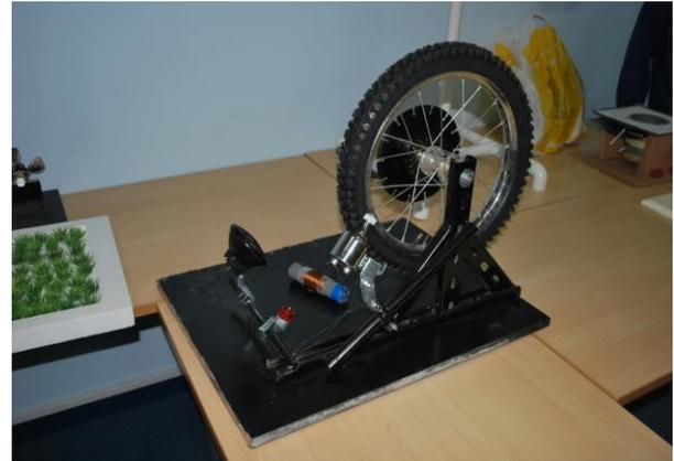
**Fig 2.** Hub Dynamo model
