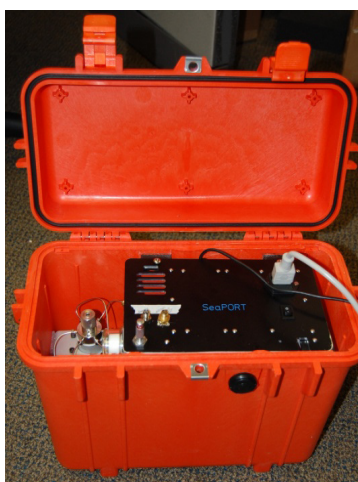
Fig 2. GC in a weather-proof case (13.5" X 7.5" X 12").
